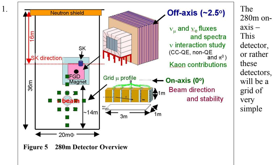
iron/scintillator sandwiches to measure the neutrino beam direction and profile. These detectors are important because the price that you pay for the benefits of an off-axis geometry is that the properties of the beam become a strong function of its direction and divergence, and these must therefore be monitored closely.
