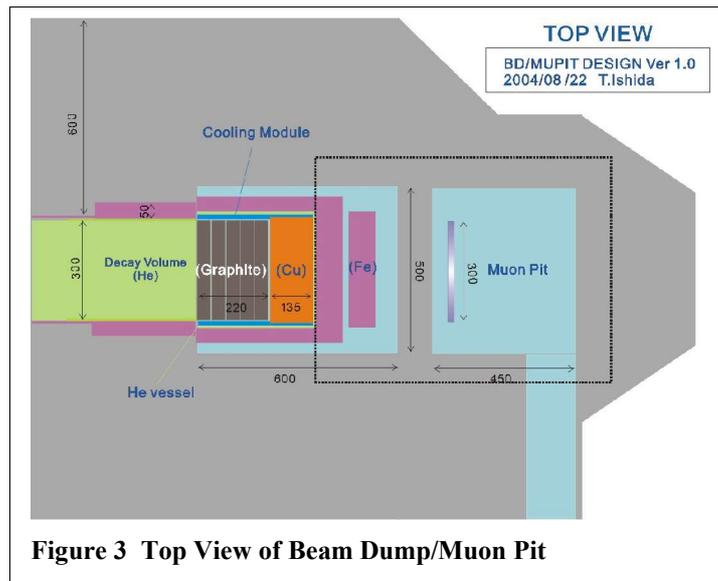
Figure 3 Top View of Beam Dump/Muon Pit
