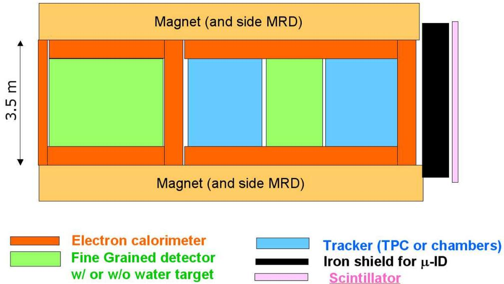
Figure 10 Block layout of the elements of the 280m off-axis detector.
