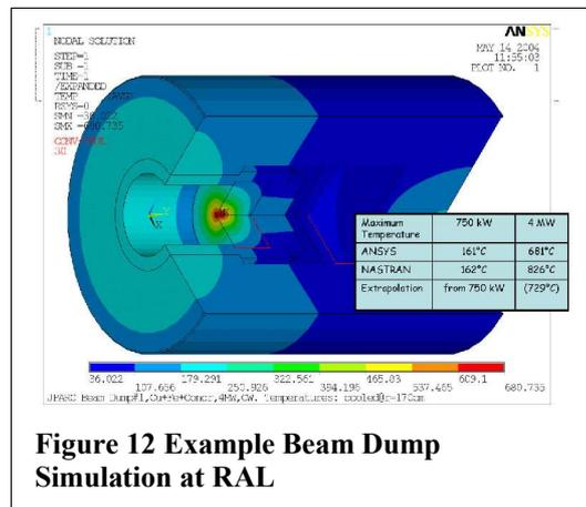
Figure 12 Example Beam Dump Simulation at RAL
