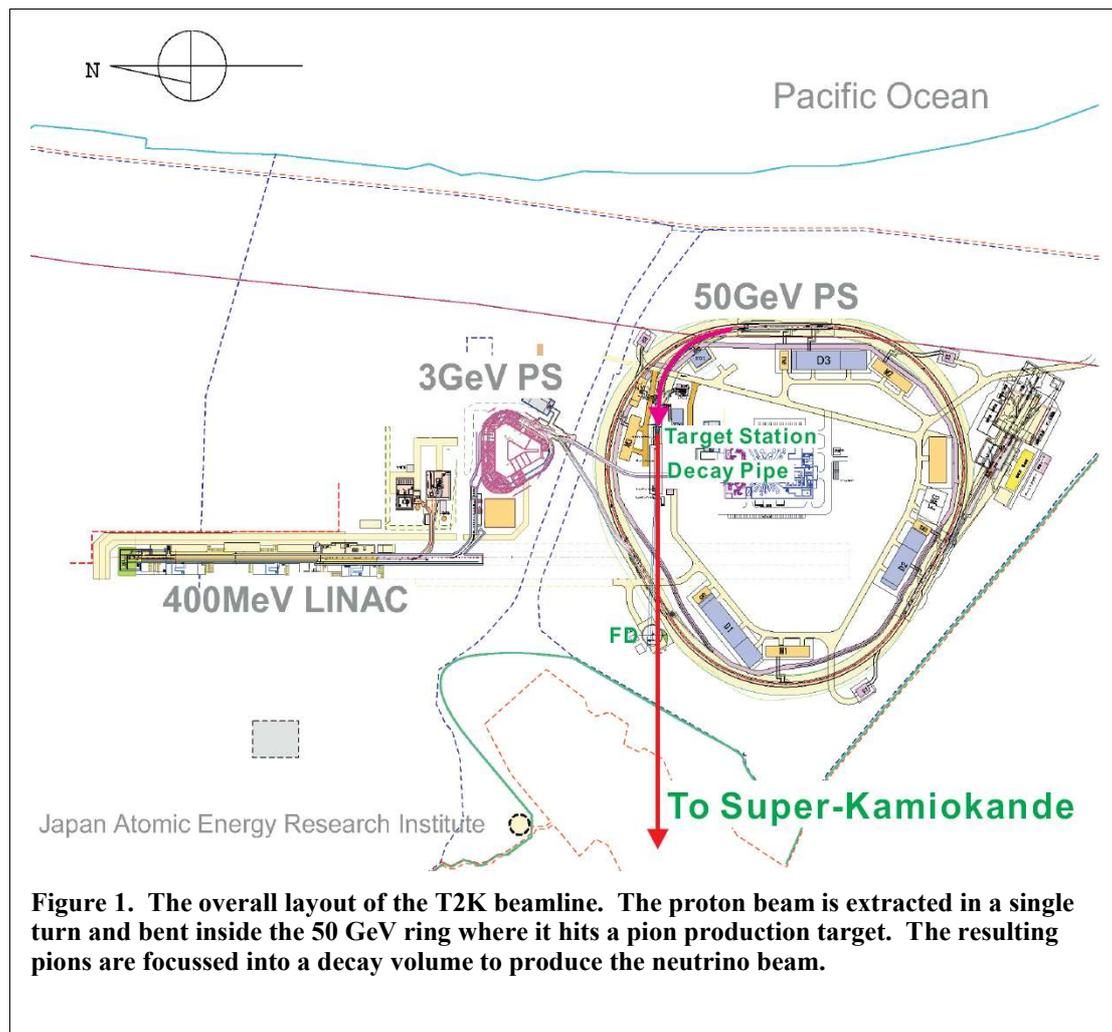
**Figure 1.** The overall layout of the T2K beamline. The proton beam is extracted in a single turn and bent inside the 50 GeV ring where it hits a pion production target. The resulting pions are focussed into a decay volume to produce the neutrino beam.
